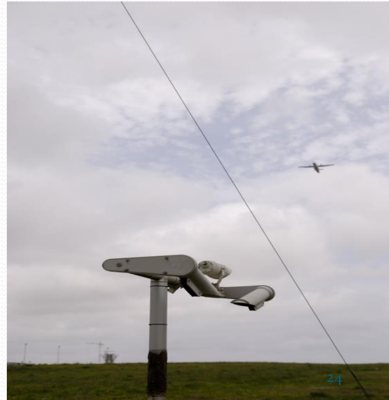
Fig. 11-4 A forward scatter visibility meter.
